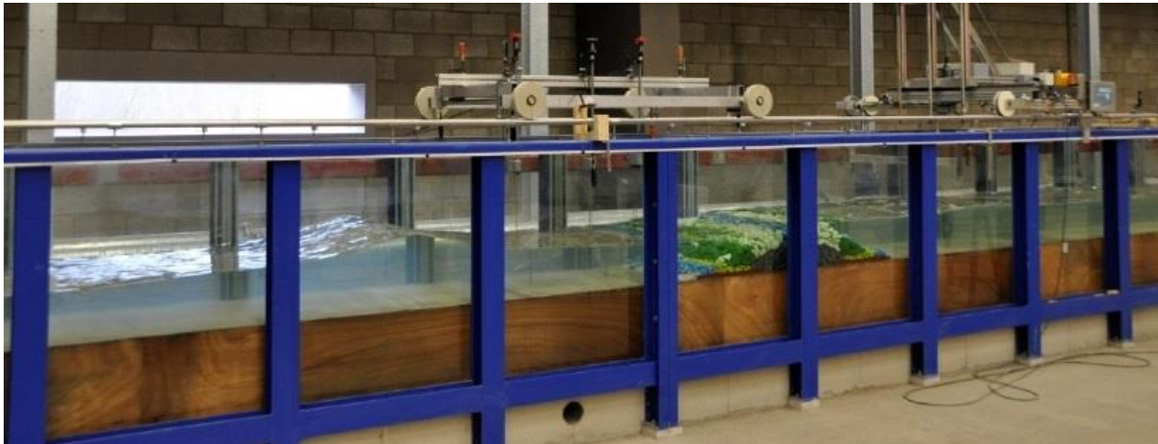
Physical model test facilities at Deltares (wave flume 1 x 1.2 x 55m)
